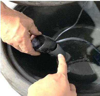
Install the cord pipe cover over the pipe and cords. This accessory helps eliminate the potential for water loss during operation.
