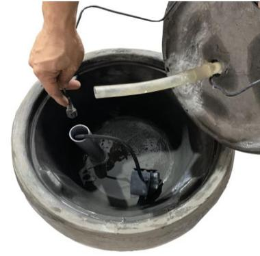
Pass the light cable down the cord pipe and retrieve it at the base.
