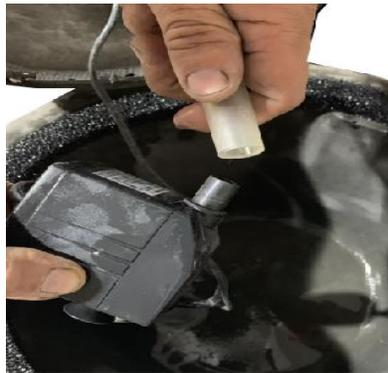
Locate the tubing and attach it to the pump. Water flow can be adjusted using the dial located on the front of the pump.
