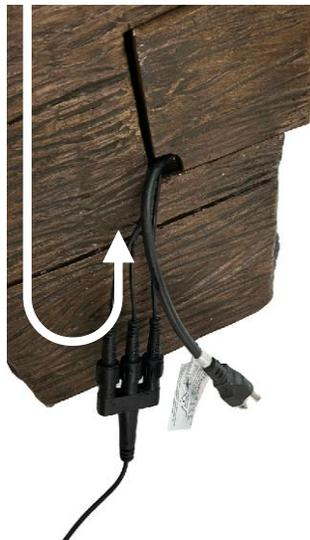
Locate and retrieve the light connection from inside the fountain. To prevent the risk of water loss, create a drip loop with the cables from the lights. Align the pump cord and light cables with the groove. Slide the pump access door in place.
