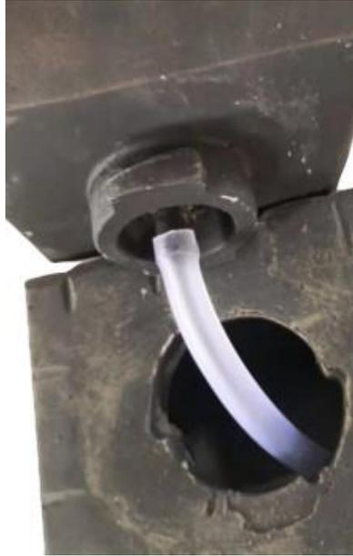
Locate the tubing and top bowl of the fountain. Attach the tubing to the fitting from the top as shown above.
