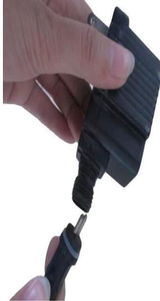
Securely attach the cord from the lights to the transformer.
