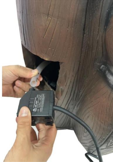
Locate the tubing and attach it to the pump. Water flow can be adjusted using the control dial on the front of the pump.
