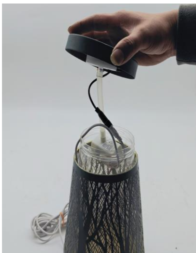
Place the pump with light cable attached inside the reservoir.
